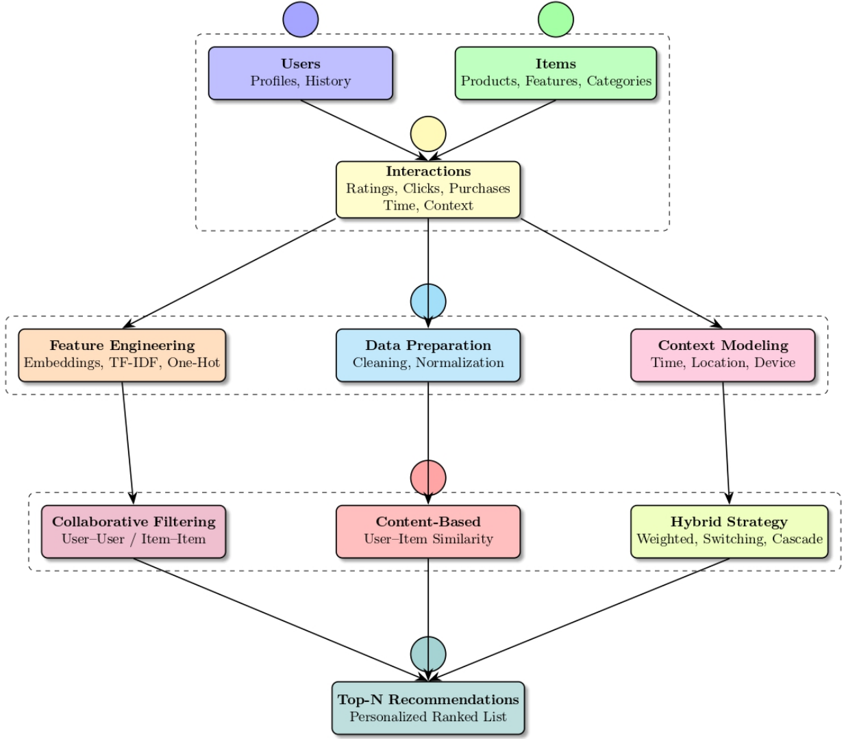
Figure 1.1: General Architecture of a Recommender System. The system integrates user and item data, interactions, preprocessing steps, and multiple recommendation algorithms to generate top-N personalized outputs.
