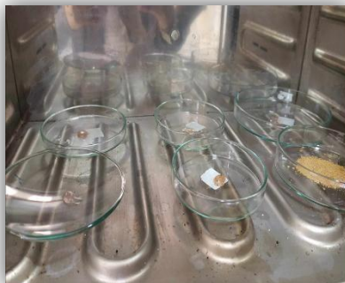
Figure 16: Determination of moisture content. (Belhani, 2024).
