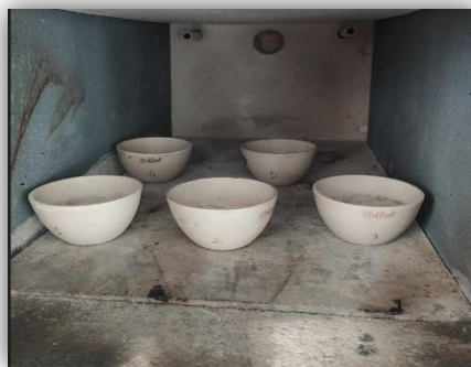
Figure 17: determination of Ash content (Belhani, 2024).
