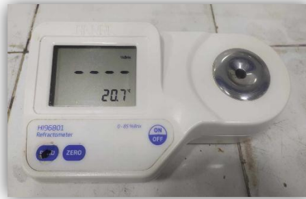
Figure 15: °Brix determination of strawberry jelly samples (Belhani, 2024).
