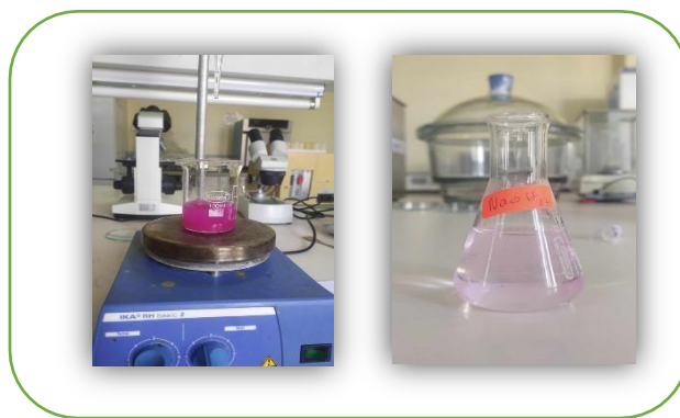
Figure 12: Determination of pectin physicochemical characteristics by titrimetric method ( Belhani, 2024 )
