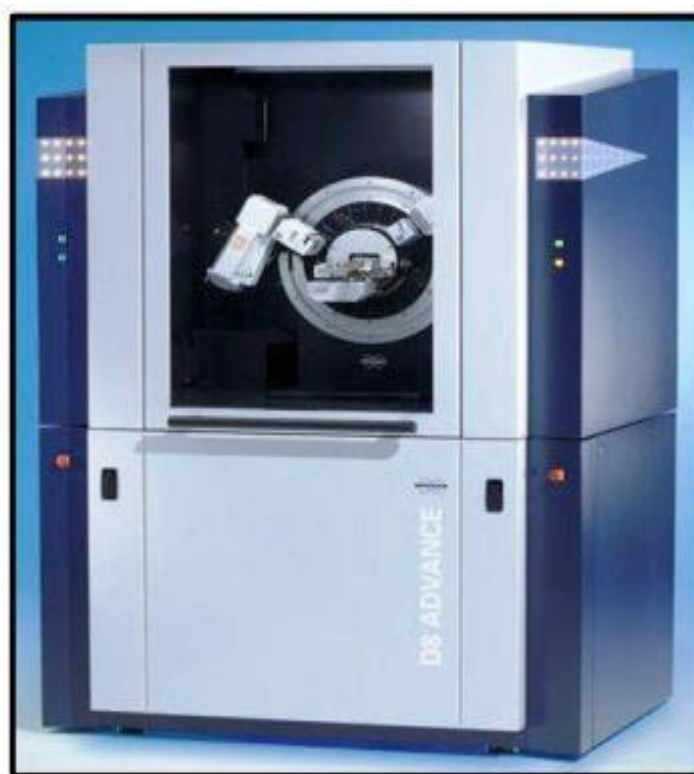
Figure II.7 : Diffractomètre Bruker D8 Advance.
