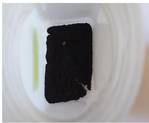
Fig.III.14: Manganese-cobalt spinel ferrite powder
