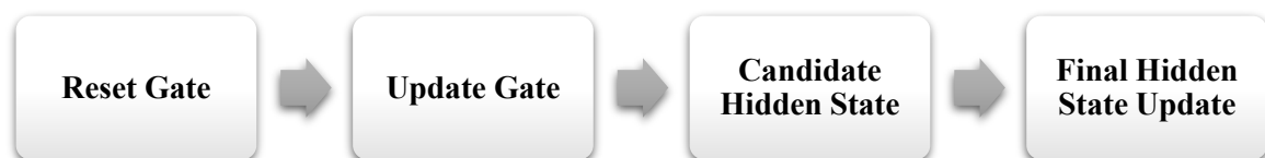
Figure 3-38: The Inner Mechanisms of a GRU.
