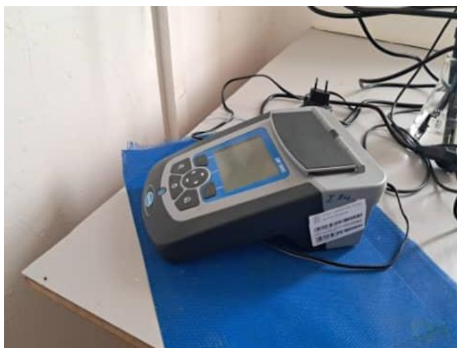
Figure 27: Spectrophotomètre HACH DR1900 (Photo Hendi Fathi 2026)
