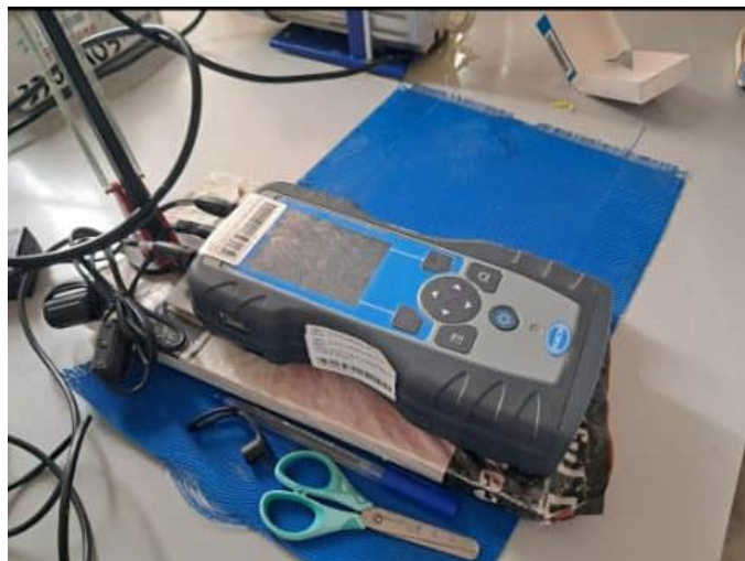
Figure 28: Multi- paramètres HACH SL1000 (photo Hendi Fathi 2026)
