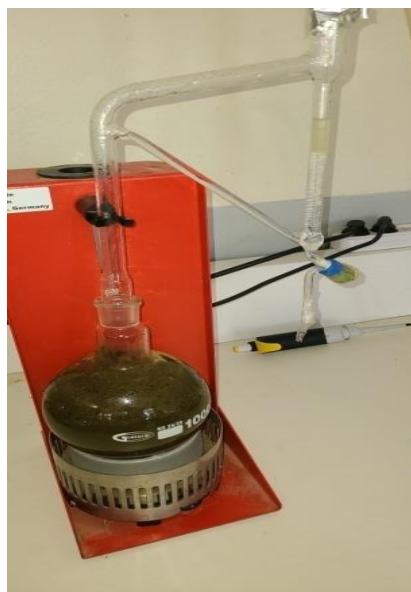
Figure 13 : Oil and water separation by density.
