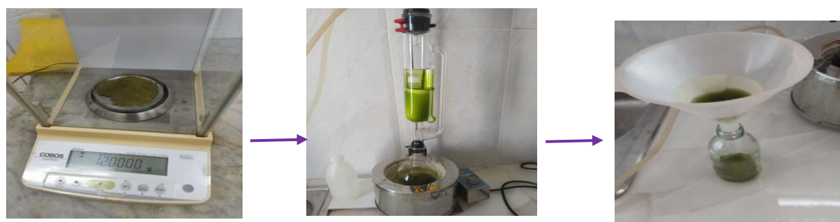
Figure II.3: preparation of concentrated methanolic extract
