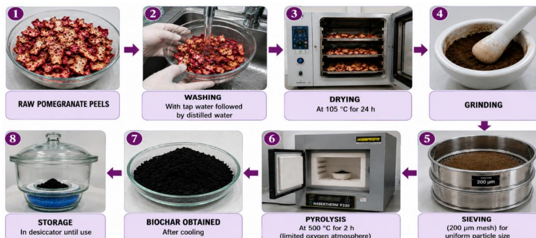
Figure II.2: Steps in the production of biochar from pomegranate peels.
