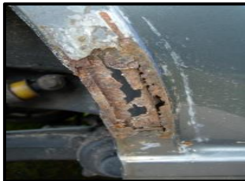
Figure I.2. La corrosion uniforme
