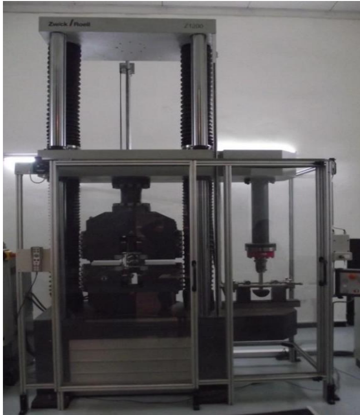
Figure III.11 : Machine de traction universelle de type Z1200 ZWICK/ROELL
