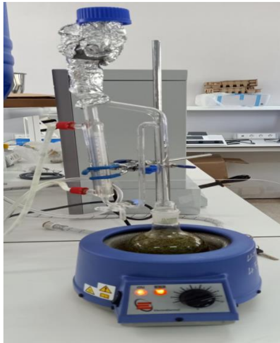
Figure II .1. Montage d'Hydro distillation (Clevenger).
