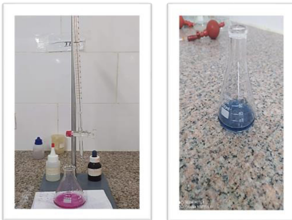
Figure 09 : Dosage de TH (BOUTELDJJI& MELLOUK, 2021).
